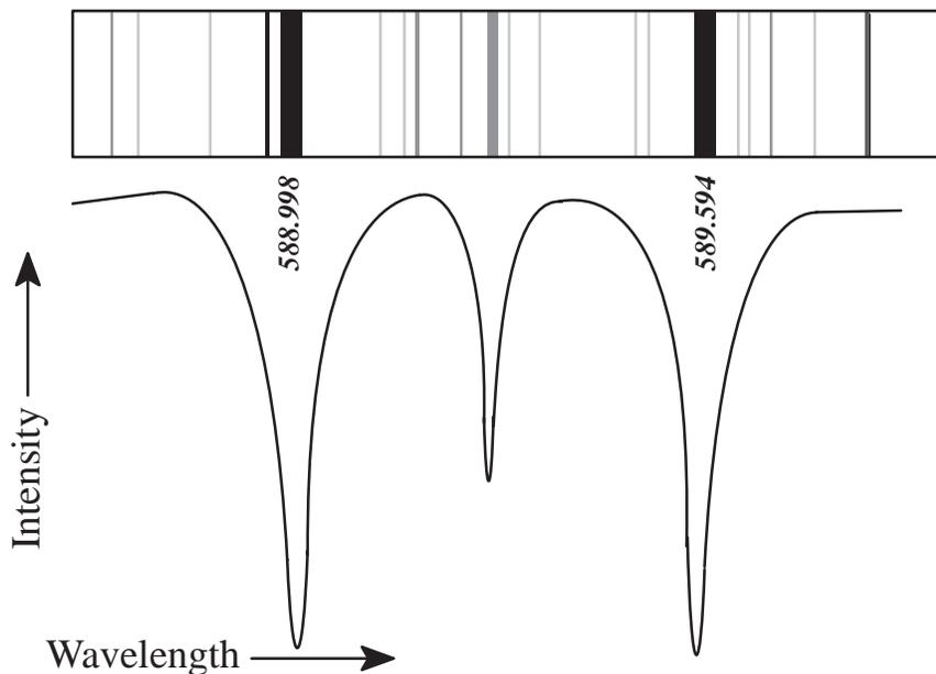
**Figure 3–5.**—Schematic of Sodium absorption from a Solar white-light spectrum. Top: The two dark absorption lines with wavelengths of 589.0 and 589.6 nanometers are produced by sodium atoms absorbing at these wavelengths. Fraunhofer observed these two lines as one, which he named the “D” line. Bottom: The same spectrum as seen on a graph of intensity versus wavelength. Each dark line appears as a drop in intensity, where light is subtracted from the continuous spectrum.
