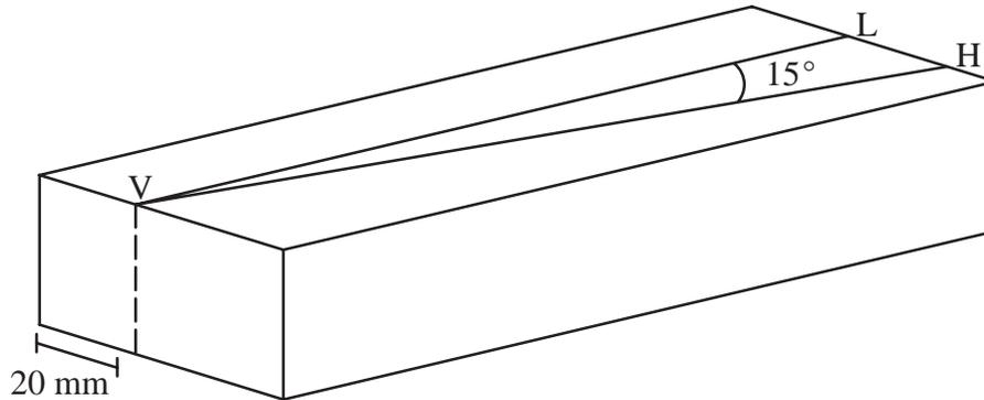
2. On the vertex end of the box cut a 10 mm square hole through the box, centered above the vertex (V) you drew and center in the end as shown:
