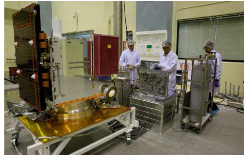
Propellant Tank Leak Test on FM 6
