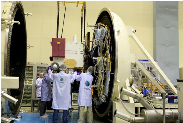
FM2 Preparation for Thermal Vacuum Testing
