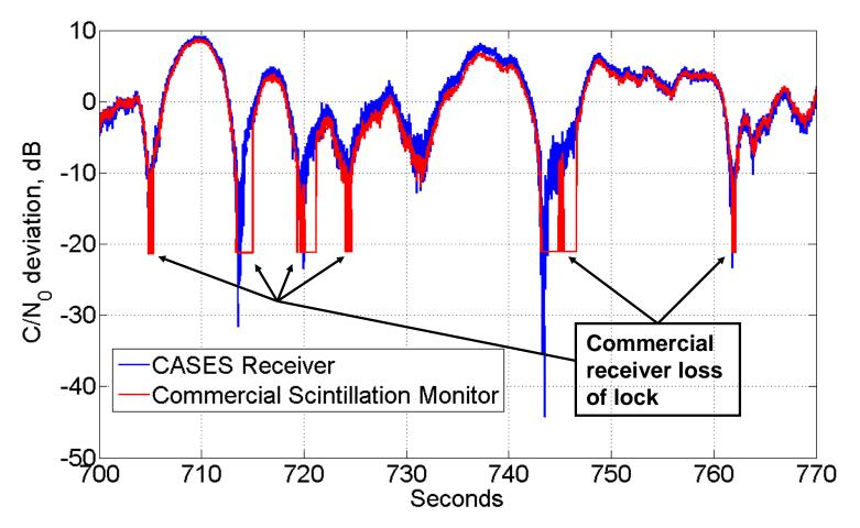
The CASES specialized tracking loop (blue trace) allows robust tracking during scintillations versus other receivers using fixed bandwidth PLL (red trace) which lose lock.
