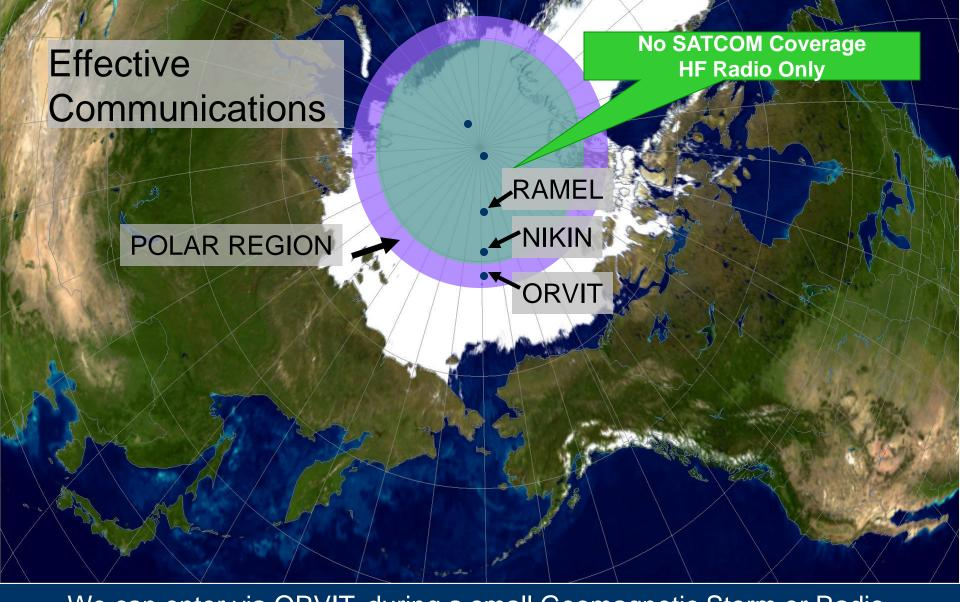
We can enter via ORVIT, during a small Geomagnetic Storm or Radio blackout because it is within SATCOM range. We will not fly any polar routes during a moderate or larger solar radiation storm due to effects on communications and possible radiation exposure.
