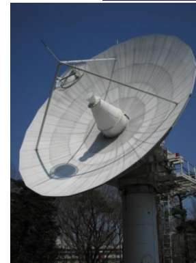
11-meter Antenna: X-band
