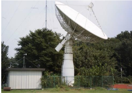
11-meter Antenna: S-band
