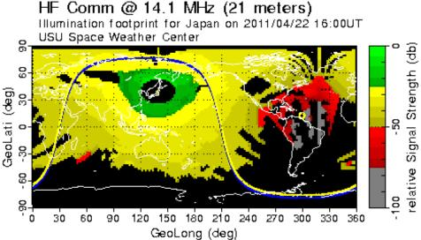
HF Comm @ 14.1 MHz (21 meters) Illumination footprint for Japan on 2011/04/22 16:00UT
