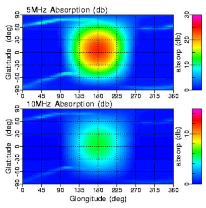
\*ABsorption BY the D and E Region of HF Signals with NORMAL Incidence
