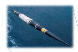
Repeaters require power, which is provided by copper conduit built into the undersea cable.
