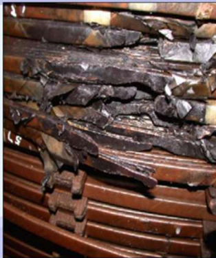
Transformer #4 HV Winding Damage
