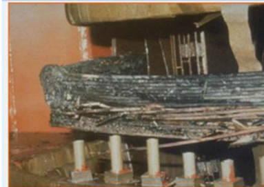
Salem GSU Unit #1 (Winding Damage)
