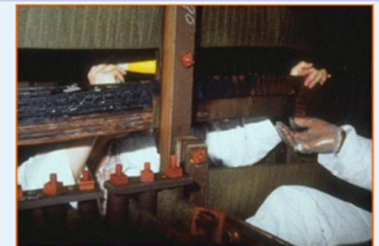
Salem GSU Unit #1 (Winding Damage)
