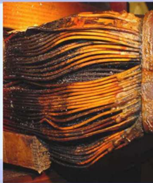
Transformer #5 Lead Overheating
